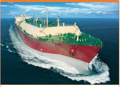
Large LNG projects typically transport LNG (gas cooled to -161°C) by ship. Although as shall be seen later SSLNG projects are transporting gas by road tanker and smaller LNG ships.
